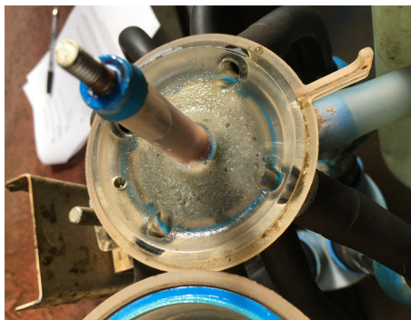
Figure 1. Inorganic (mineral) and organic (milk) deposits on claw bowl surfaces
