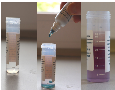
Figure 2. Fill tube with 20 ml of water; add one drop of KW15 at a time, mixing between drops; number of drops required to change colour (red to blue) indicates hardness. Hardness equals (drops KW15 used) x 10
